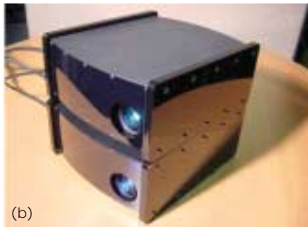
4 The FLEA: (a) 120-Hz stereo DLP projector; (b) stacked for two-person collaborative use.
