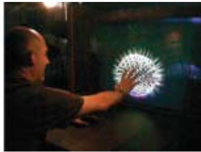
(a) (b) (c) 3 Creating a virtual workspace: (a) a holographic diffuser allows simultaneous viewing of projected and real images; (b) shared virtual workspace projected between collaborating users; and (c) four-person configuration.
