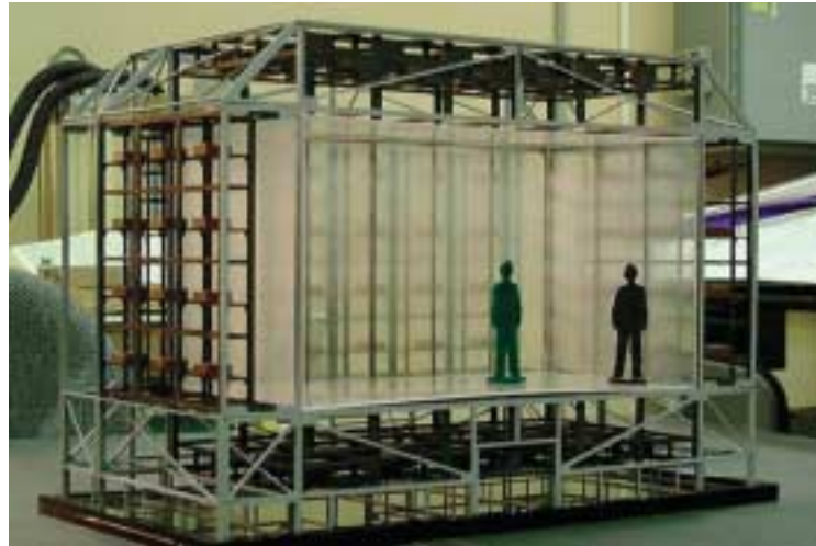
5 Gazillion-pixel array of stereo projectors showing small footprint and overall form
